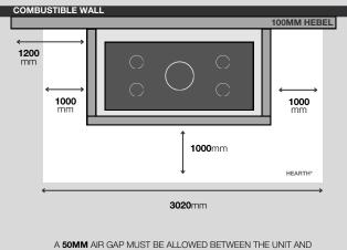
50MM AIR GAP MUST BE ALLOWED BETWEEN THE UNIT AND ENCLOSURE
