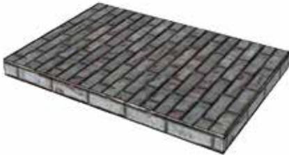
Lay a masonry base, minimum 150mm thick (ie. Solid bricks). The base should be laid on an adequate ground capable of supporting its weight.
